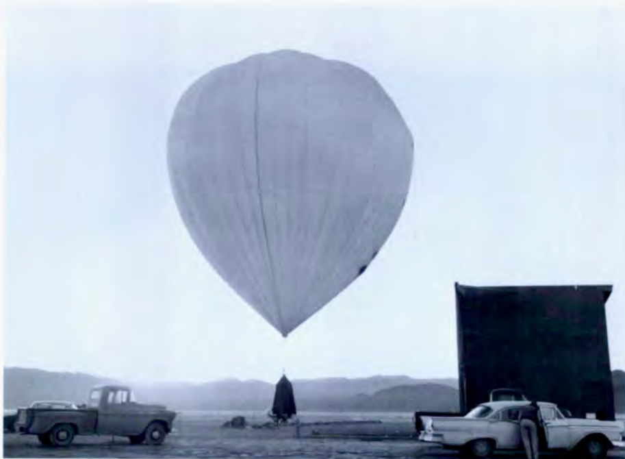
This photo of a balloon-carried test configuration was taken around 1957. The device is suspended from the balloon and the balloon is tethered to the ground by steel cables. With the balloon at the desired altitude (perhaps 1500 feet) the device was fired by sending electrical signals through the firing cables that connected the device with the firing system on the ground.
